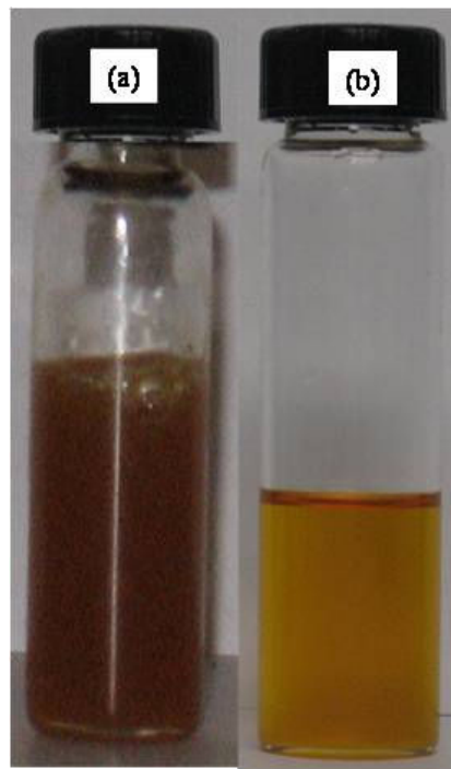
Figure 4.16. TG (a) and biodiesel (b) obtained from feather meal.
