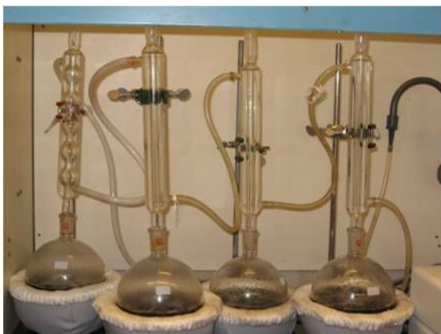
Figure 3.1. Experimental setup for oil extraction from spent coffee grounds (reflux with organic solvents).
