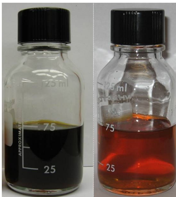
Figure 4.9. Coffee oil and biodiesel produced from spent coffee grounds.
