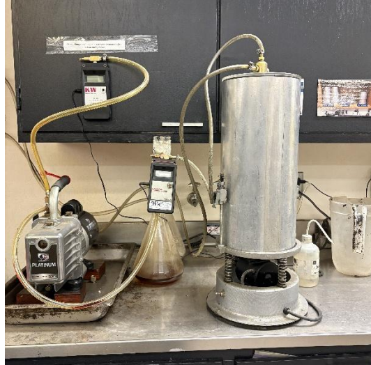
Figure 17: Vacuum apparatus for T283
