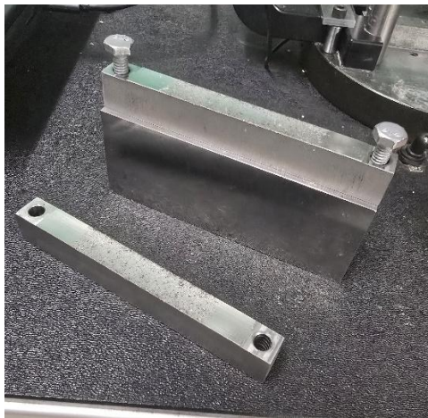
Figure 11: Loading strip modification
