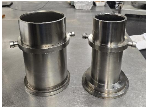
Figure 6: Compaction molds for 150 mm and 100 mm
