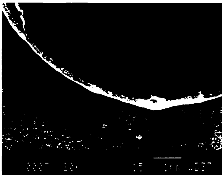
Figure 32 SEM image in backscattered electrons of the reaction zone on the graphite rod with magnification 15X.
