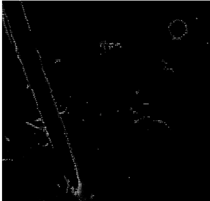
Figure 3. A rasterized cross section of a point cloud 1.37 m above ground.
