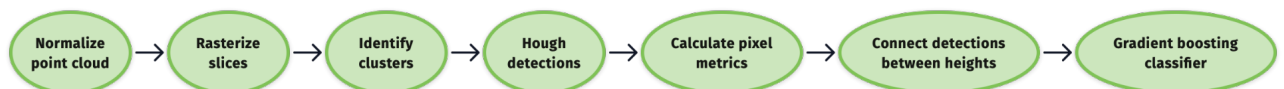
Figure 6. The seven steps of the Discovertree approach. The first step is to classify the point cloud so points can be subset by height above ground. Slices of the point cloud are rasterized at multiple height levels, then divided into clusters. Hough transforms are parameterized for each region, then a series of pixel metrics are calculated for each Hough detection. The detections are connected between different height layers and finally fed into a gradient boosting classifier.
