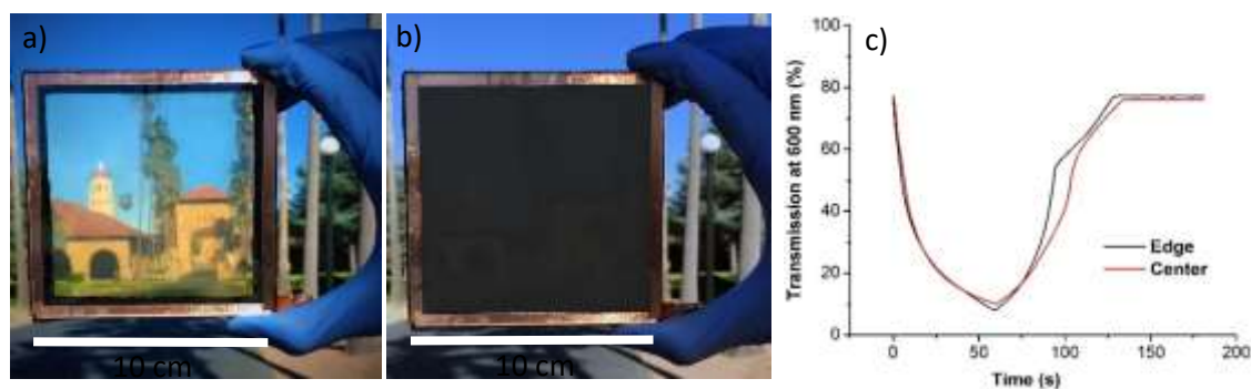
Figure 2.6. 100 cm 2 Hybrid Dynamic Windows. Photographs of a 100 cm 2 dynamic window after 0 s ( a ) and 120 s ( b ) of metal electrodeposition using a Pt-modified ITO on glass working electrode and a LiNiO x on ITO on glass counter electrode. c , Transmission at 600 nm through the edge (black) and the center (red) of the window during switching at -2.5 V for 60 s followed by 0 V for 120 s.
