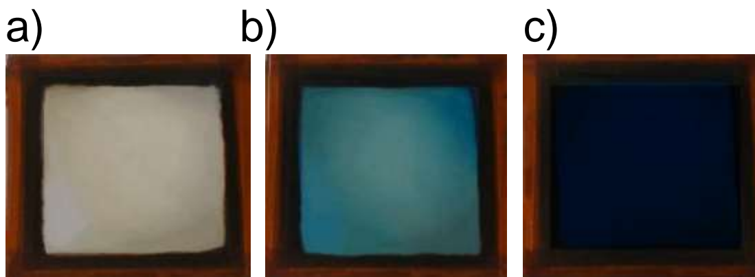
Figure 5.3. Photographs of a 25 cm 2 metal-based hybrid dynamic window with a Prussian blue counter electrode during switching at -2 V for 0 s (a), 1 s (b), and 3 s (c).
