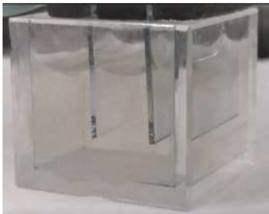
Supporting Figure 12.4.7. Photographs of a 2 cm 2 with a Pt-modified ITO on glass working electrode, a Prussian blue on ITO on glass counter electrode formed using 6 minutes of electrodeposition switching at -2 V for 0 s (a) and 3 s (b) in a liquid Bi electrolyte.
