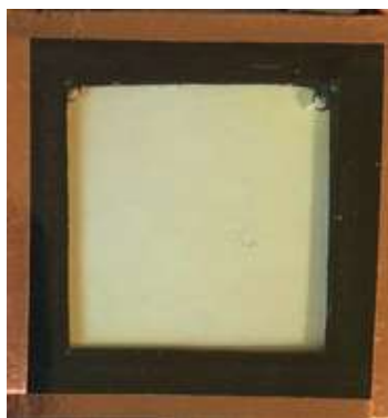
Supporting Figure 12.1.11: Photograph of a 25 cm 2 dynamic window utilizing an unmodified ITO counter electrode. Following 10 complete cycles of -2.5V for 30 s and 0V for 60 s, the device turns yellow due to the formation of Br 3 - in the electrolyte.
