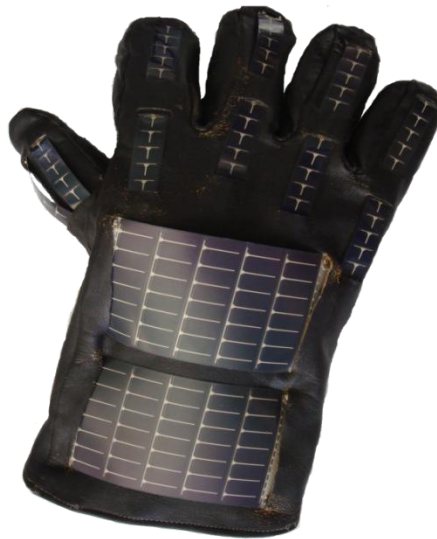
Figure 7: Completed GreenGlove Prototype.
