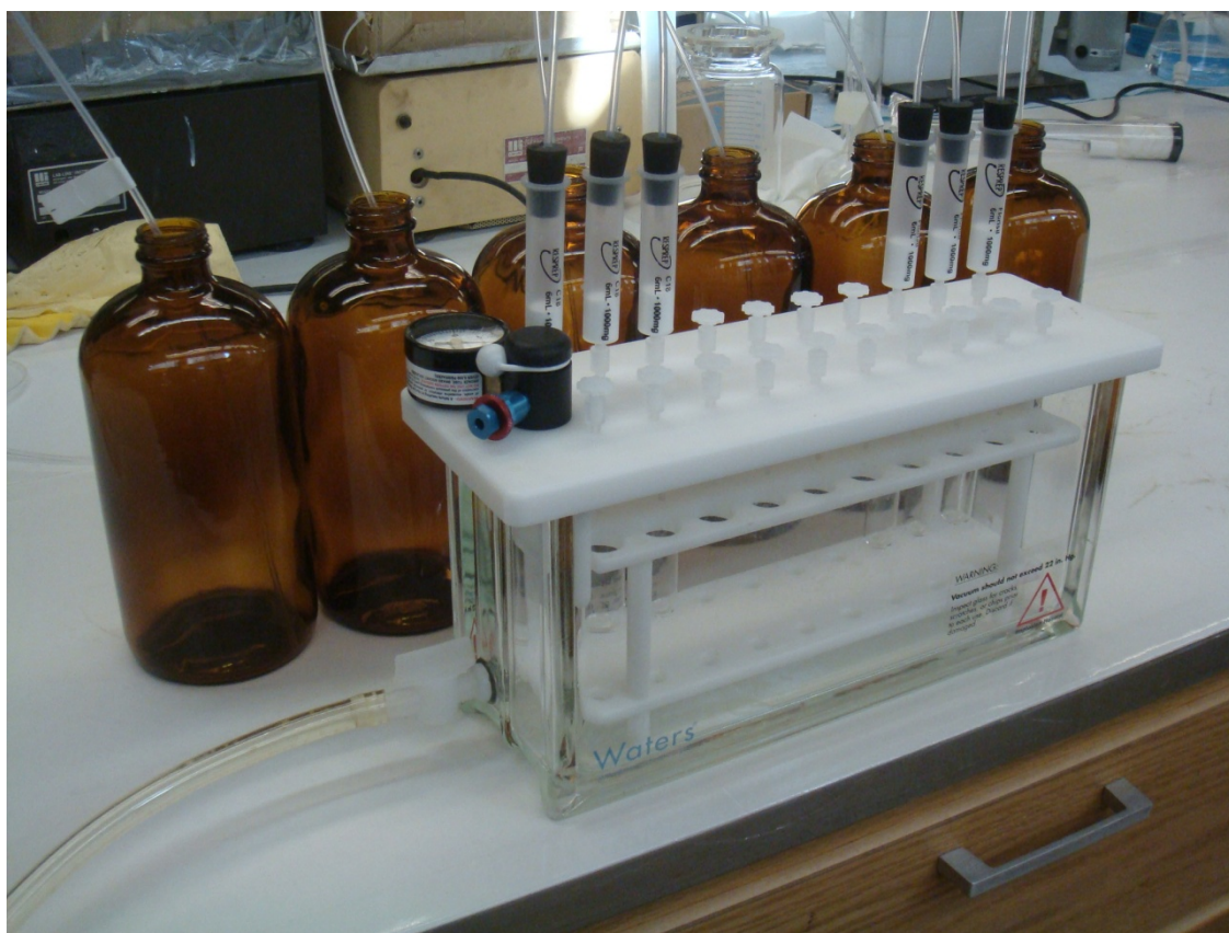
Figure 2-1: Sample set up with collection bottles, cartridges and vacuum extraction manifold
