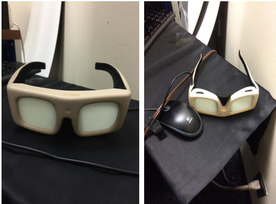
Figure 5. The PLATO goggles worn by participants during the Training phase. The goggles include computer-controlled LCD panels within a plastic frame. The goggles were used to control the exposure duration of the stimuli during each trial. Participants wore these goggles during the Training phase of the experiment (which involved the presentation of real food items).
