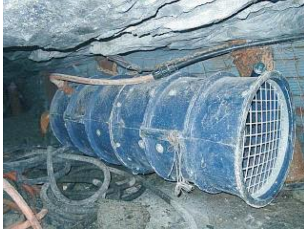
Figure 4: An experimental cooling-coil spot cooler (Biffi, Plessis, & Marx, 2005)
