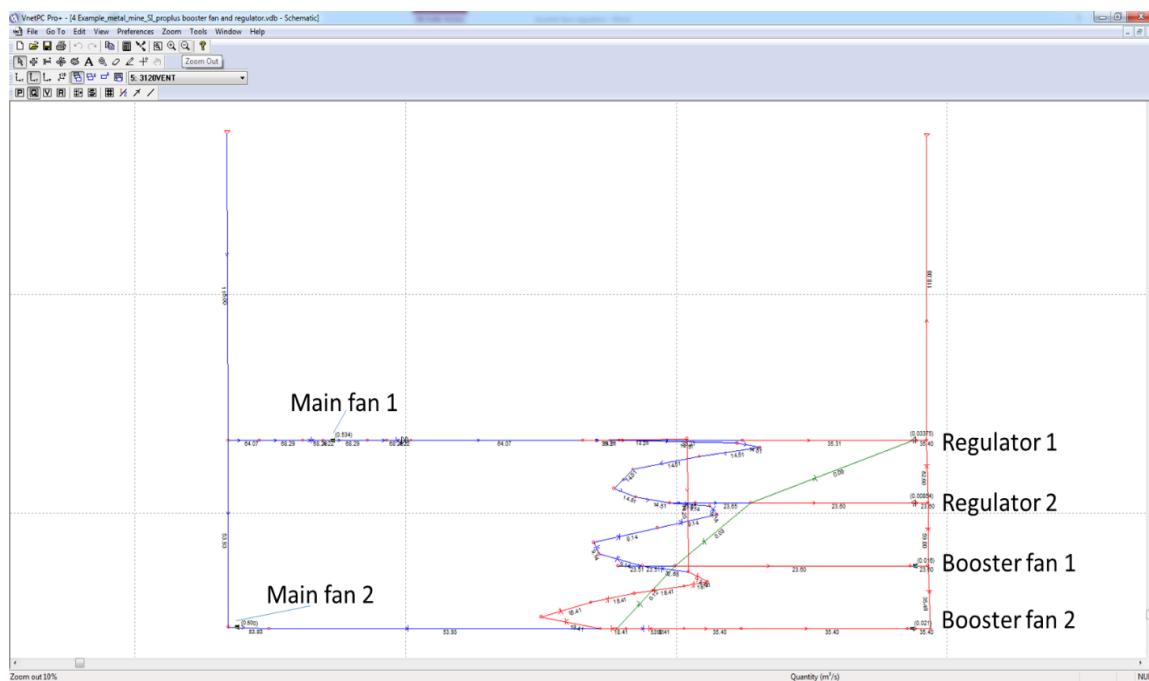
Figure 3.3 2D Layout of Mine Example 1 – Scenario 3
