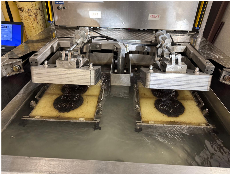
Figure 13. Hamburg Wheel Track Machine Setup Before Testing.
