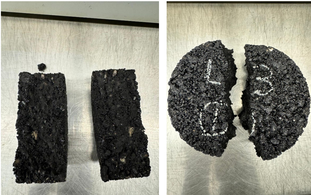
Figure 17. Specimen with Cracking Surface after the IDEAL-CT Testing.
