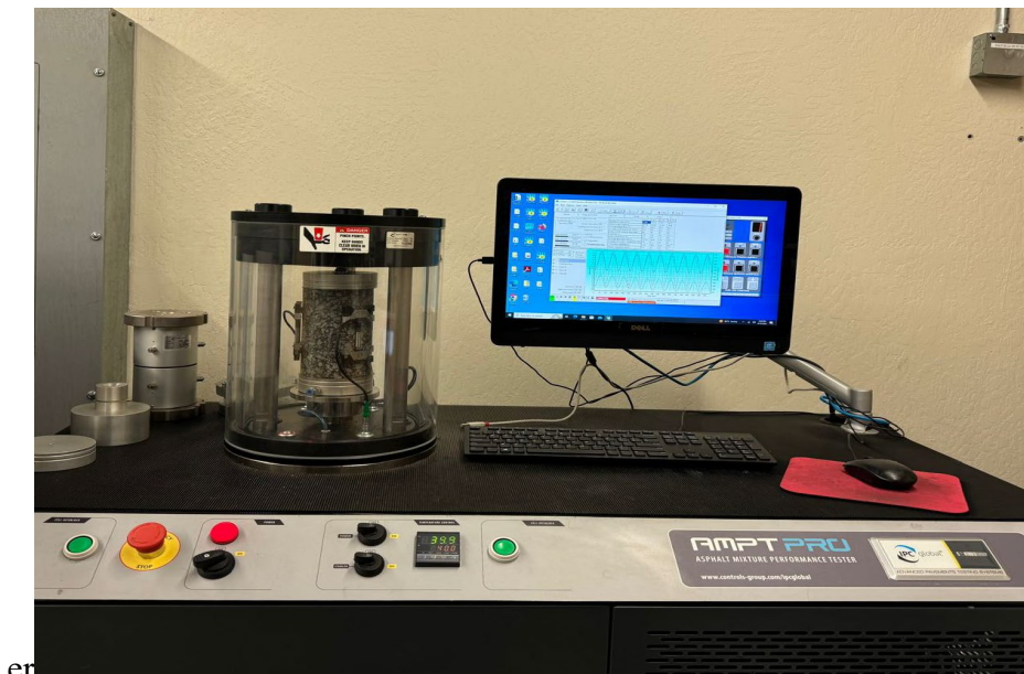
Figure 11. Dynamic Modulus Test Setup.
