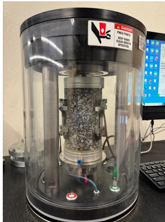
Figure 12. Dynamic Modulus Test Specimen Inside the Chamber.
