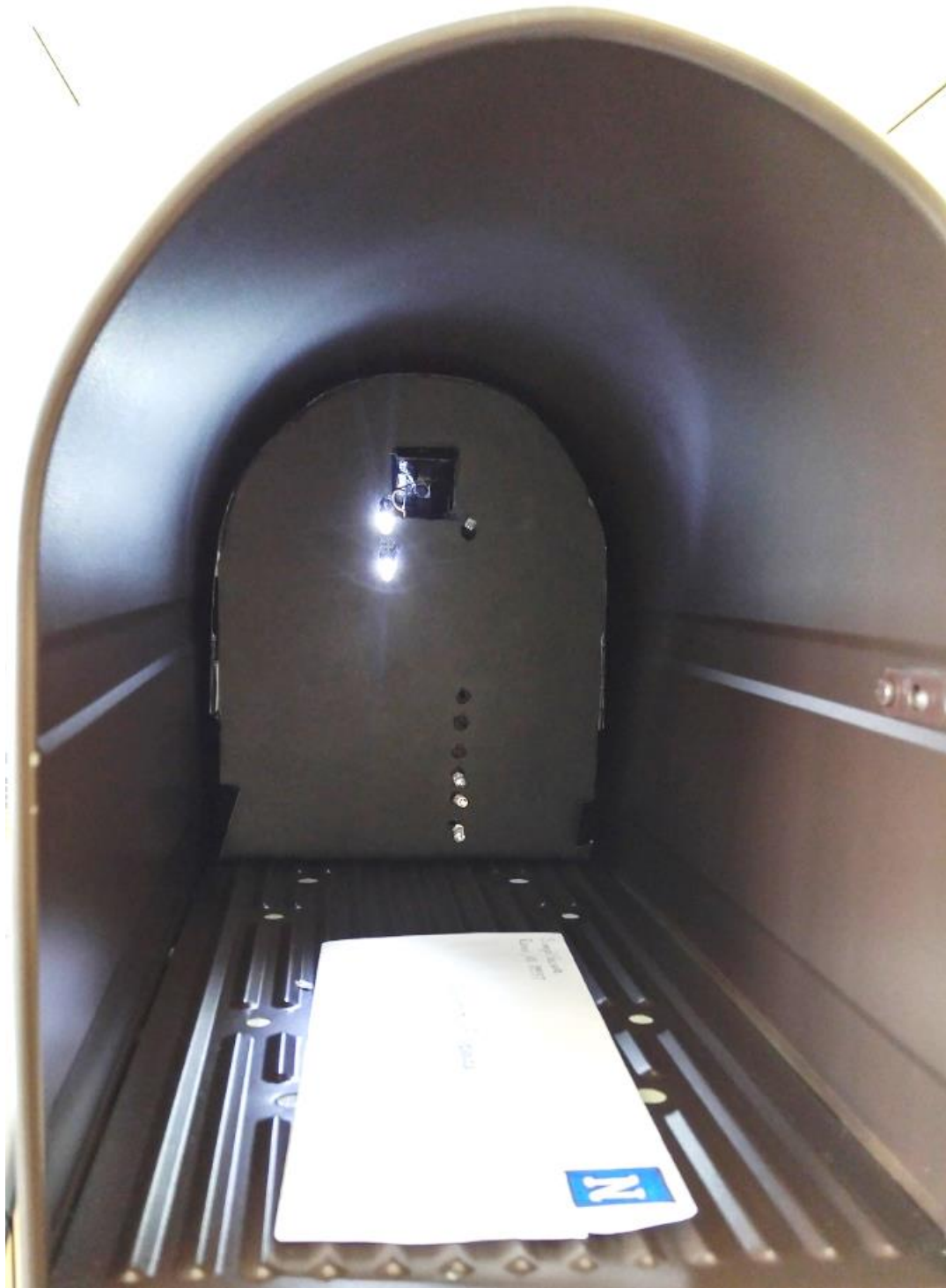
Figure 8. MailSnap turns on the white LEDs to produce a high quality photo.
