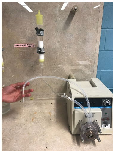
Figure 8: Cation chromatography column and pump setup.
