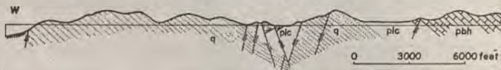
FIGURE 4—Cross-section of the south end of the Groom Range. Valley is to the left; q is Prospect Mountain quartzite; plc is Pioche shale, Lyndon limestone, and Chisholm shale; pbh is Peaslee limestone, Burrows dolomite, and Highland Peak formation.
