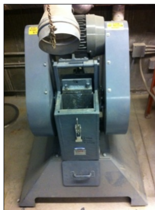
Figure 15. First Stage Jaw Crusher
