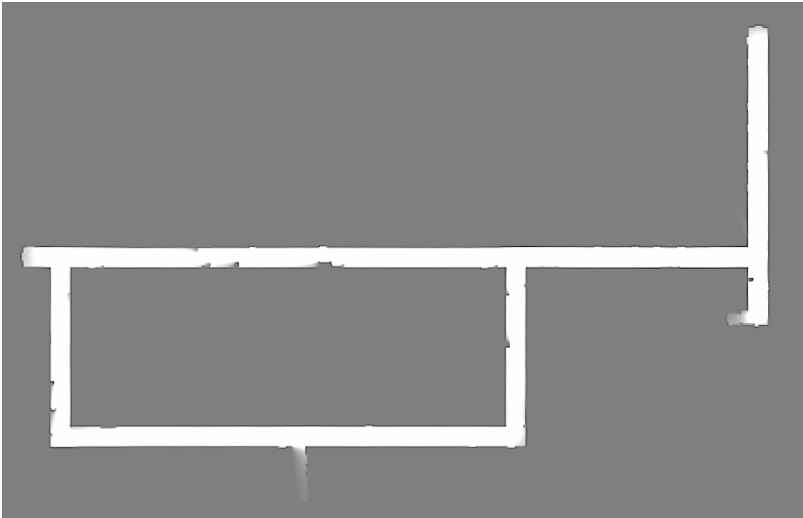
Figure III-35: Modified mapping results using a particle filter with 20 particles.
