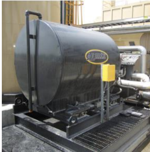
Figure 11. Skid-mounted Calibration Tank[9].
