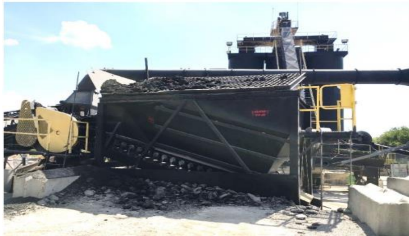
Figure 5. Cold Feed Bin with Scalping Screens to Remove Clumps[3].
