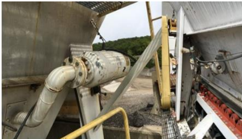
Figure 5. Cold Feed Bin with Scalping Screens to Remove Clumps[3].
