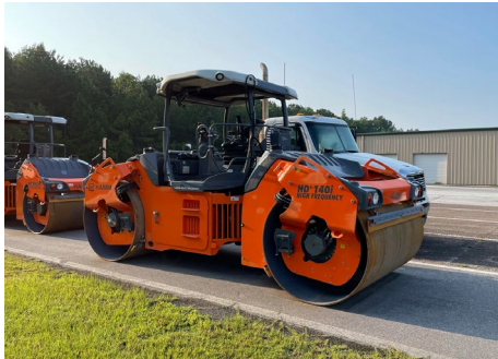
Figure 13. Intelligent Compaction Roller (Photo Credit: Jason Nelson).
