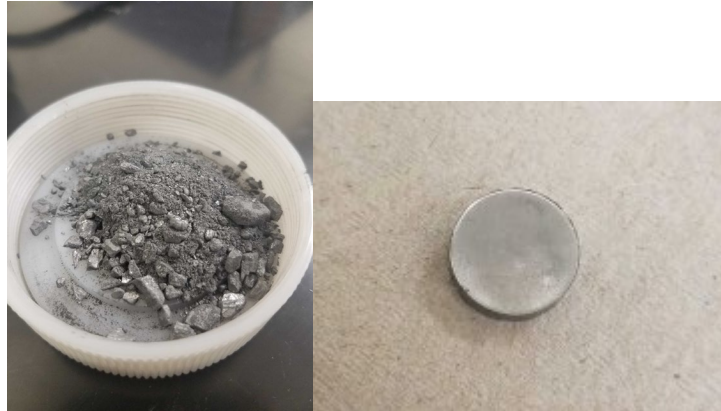
Fig. 7: Images of GST powder before grinding and ball milling process (left) and fabricated pellet (GST-4) as a result of the cold sintering press (right).
