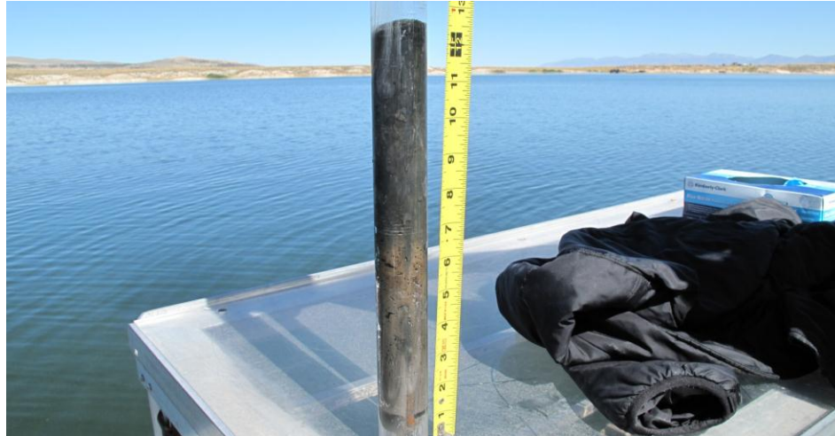
Figure 11. Image of SFH Reservoir gravity core sample collected on September 23 rd , 2009 (tape-measure values are in inches).
