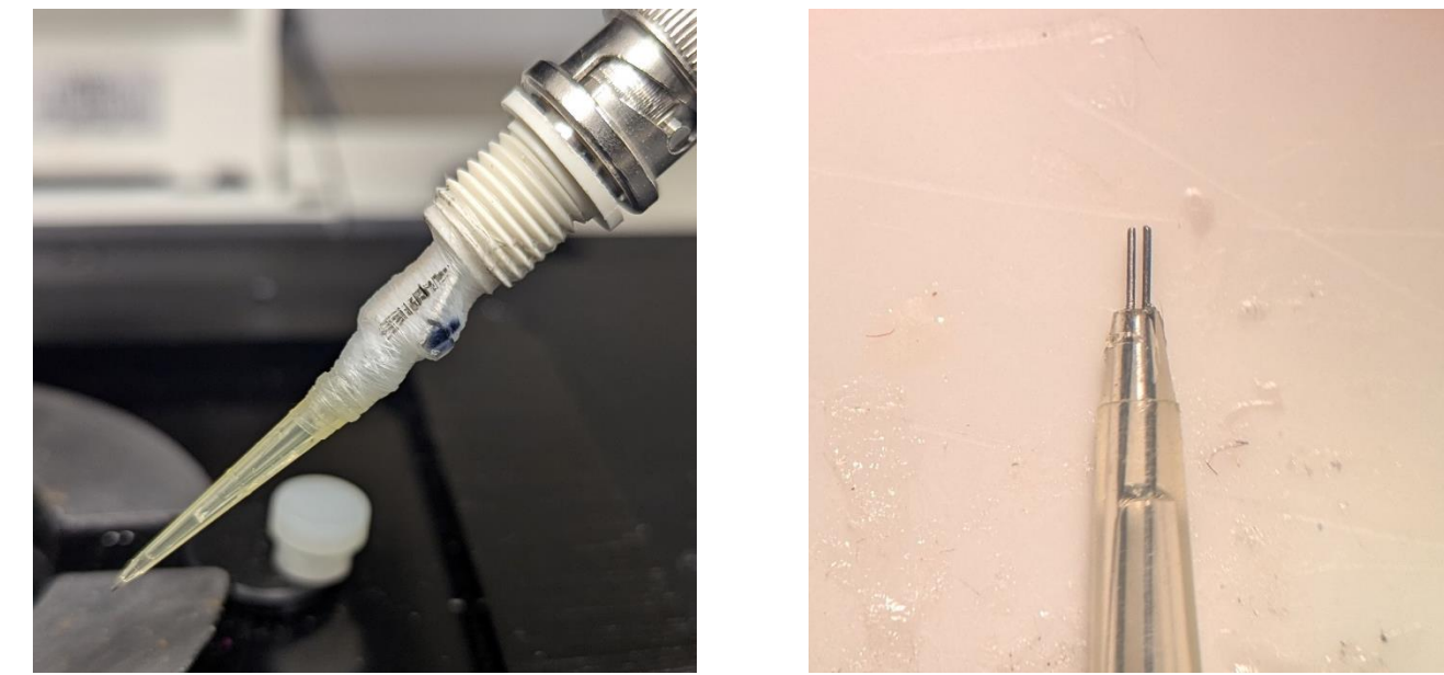
Fig. 2. (Left): A complete custom-fabricated electrode, held in place by a micromanipulator. (Right): 3X view of the tungsten rod tips of a custom-fabricated electrode.
