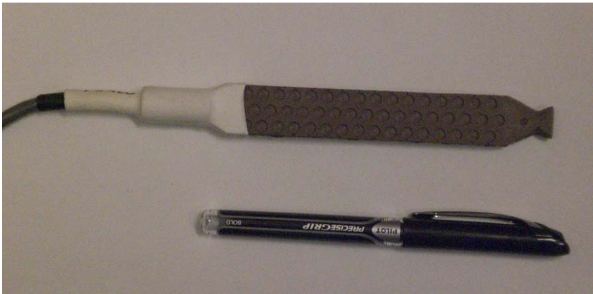
Figure 3-3: Concrete Strain Gage
