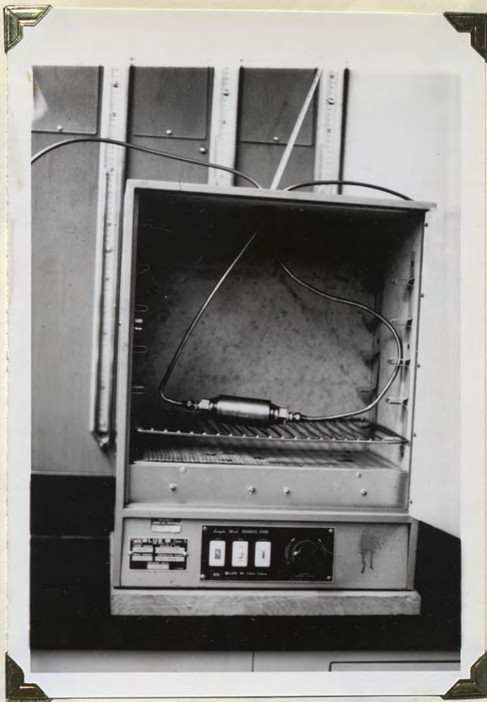
Figure 14 - The sample holder, containing the disk, shown within the oven.
