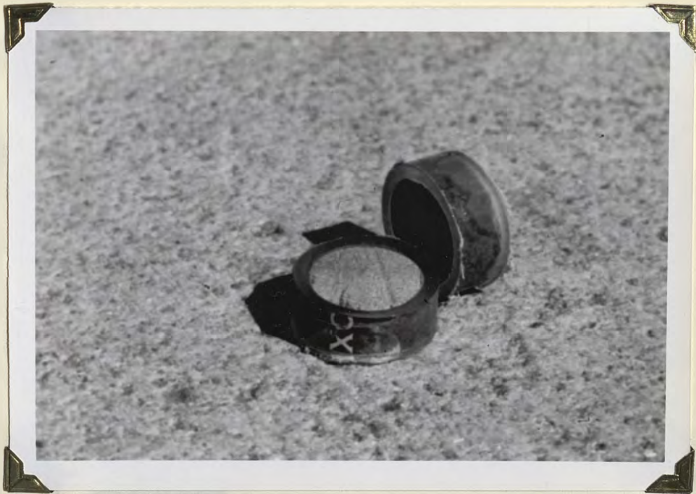
Figure 13 - Disks of sandstone, sheathed with polyethylene.
