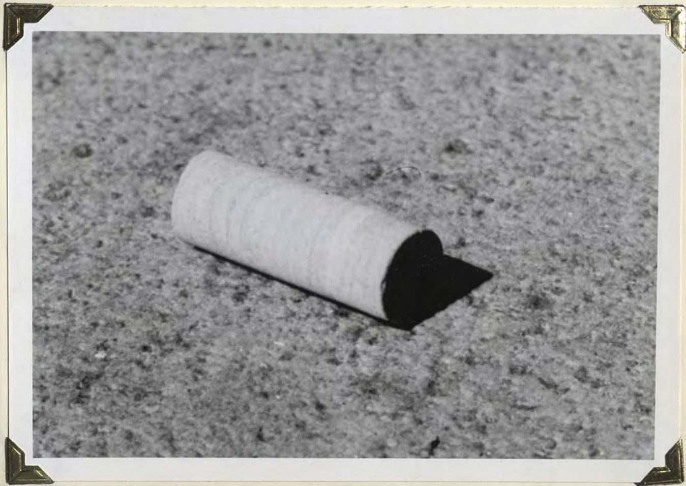
Figure 10 - One of the core samples obtained from the drilling.
