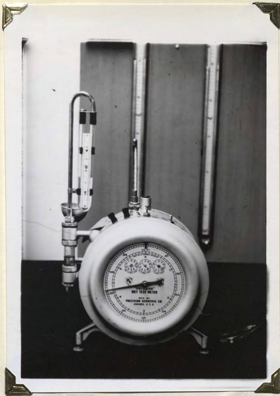
Figure 17 - The wet test meter, used to measure the volume of the air passing through the sample in time t .
