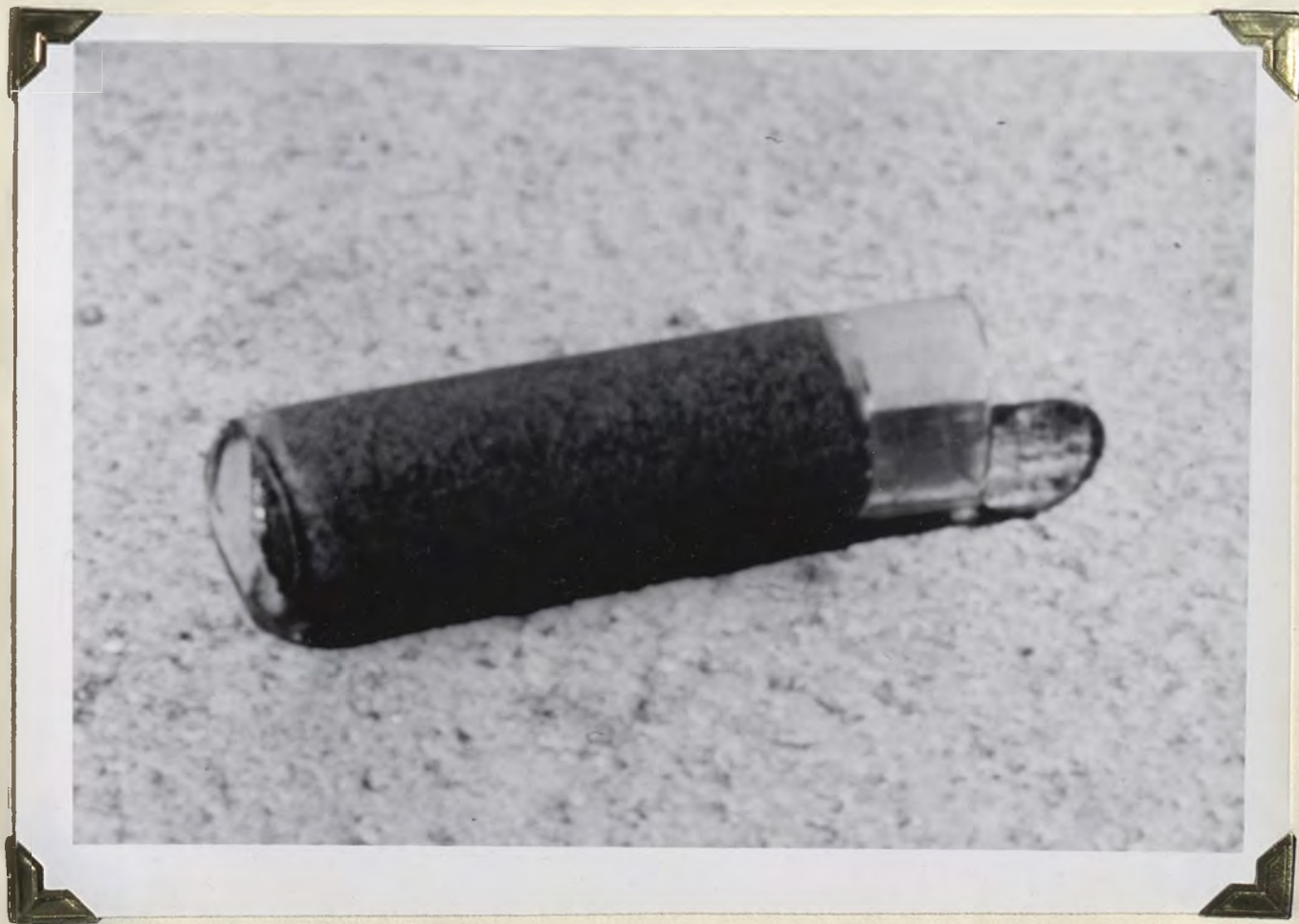
Figure 11 - One of the cores, inserted into polyethylene sheathing.
