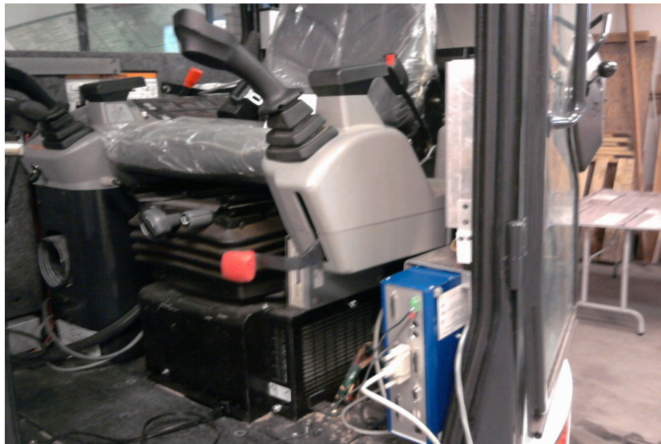
Figure 12: Control computer installed in the cab of Bobcat 435 excavator.
