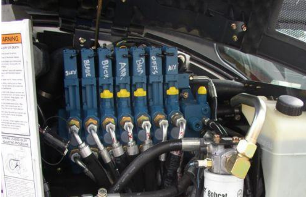
Figure 9: Electro-hydraulic valves installed on Bobcat 435 excavator
