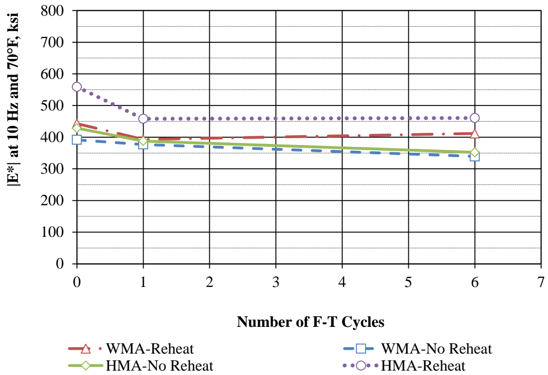
Figure 20 |E*| of Field Mixtures at 70°F as a Function of F-T Cycles.
