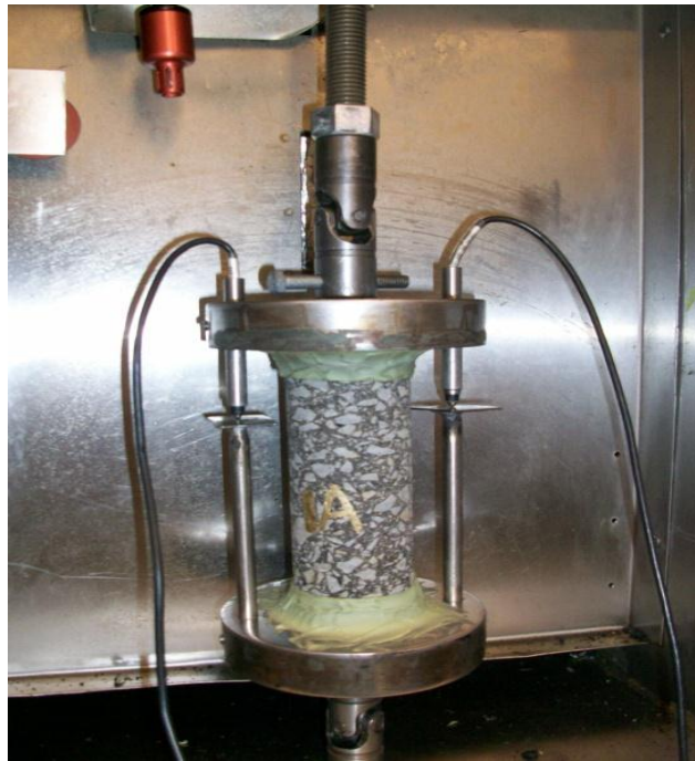
Figure 18 Prepared TSRST Sample in Testing Chamber.
