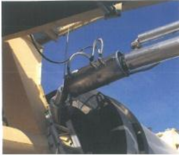
Figure 5 Maxam AQUABlack™ WMA System Unit Installed on a Drum Mix Plant.
