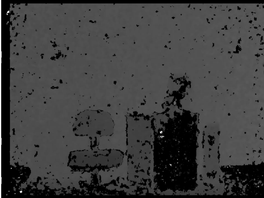
Figure 3.2: Depth image obtained from our sensor before any filtering operations are performed. Black spots show areas of missing depth. Very bright spots show incorrect depth measurements.
