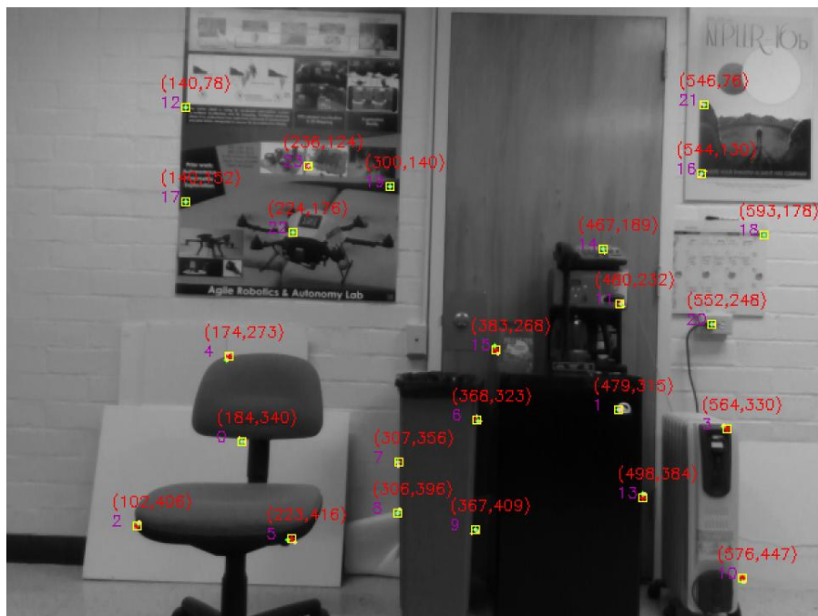
Figure 3.9: An instance of 25 best selected features from the combined score image that satisfy the selection criteria. Comparing the location of selected features to the Visual and Depth Score images it can be observed that the selected features originate from both domains.
