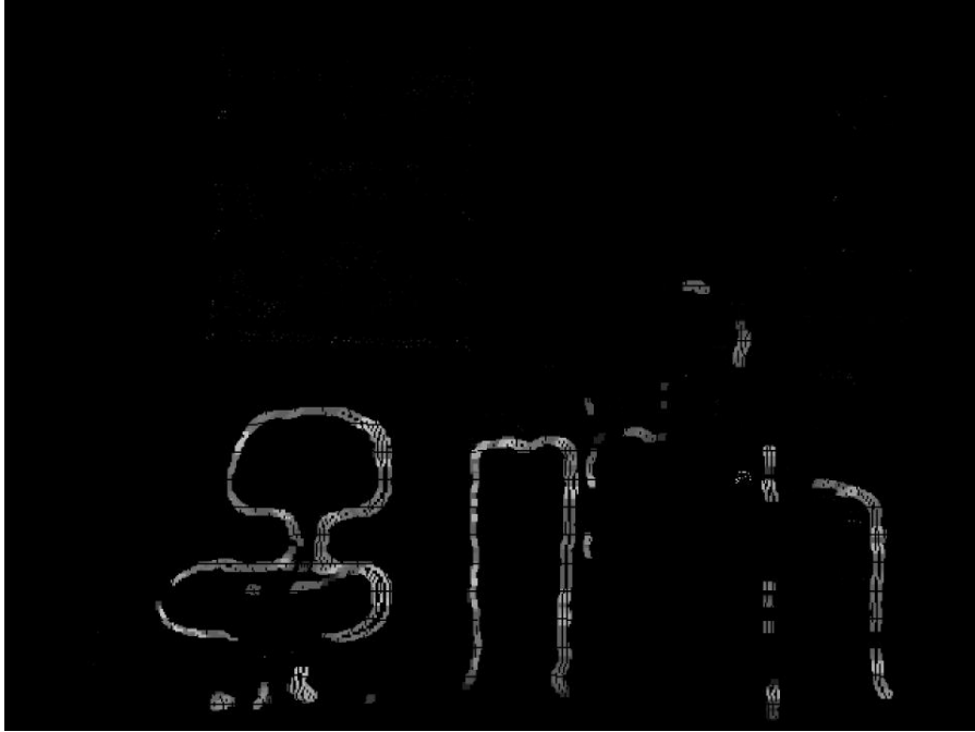
Figure 3.8: Final combined visual and depth score image to be used for final feature selection.
