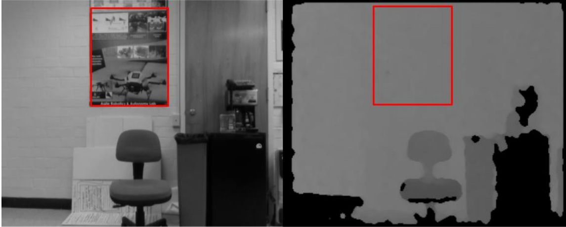
Figure 1.1: Visual and Depth images of a scene taken in good illumination conditions are shown side-by-side. The poster on the wall provides rich texture information in visual domain but does not provide any structural information in depth domain.
