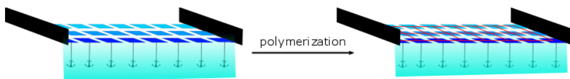
Figure 1.15. Polymerization using an LB trough. Monomers depicted by squares are compressed into a monolayer by the black barriers. Anchors represent hydrophilic groups which keep the monomers consistent in orientation with respect to each other. Polymerization indicated by red lines between monomers. 24
