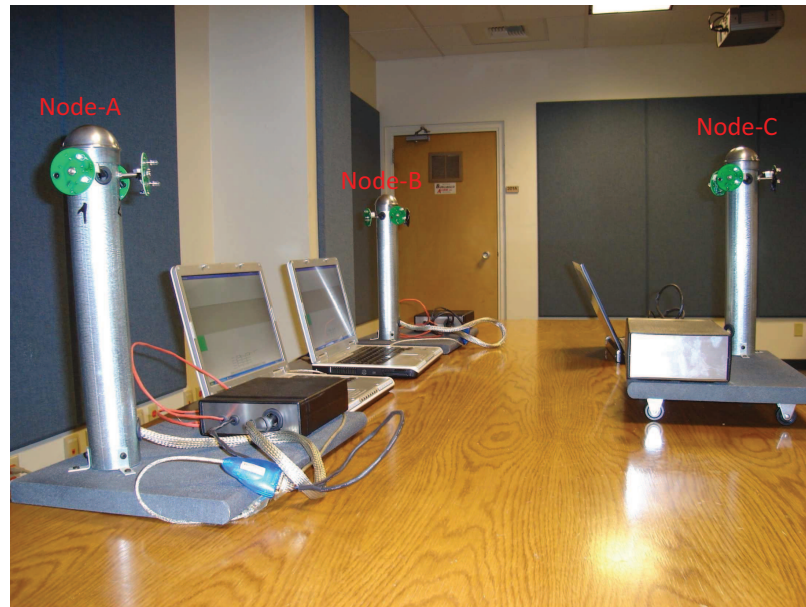
Figure 5.9: Indoor experiment setup: 3 laptops (collinear placement), each with a 3 transceiver optical antenna.
