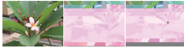
Figure 5.21: Original image and received image files for image file transfer in half duplex mode. The very left picture represents the original image file and following images are received images at Node-B and Node-C accordingly.
