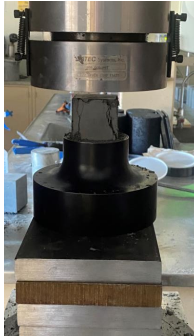
Figure 22. Compressive strength test of 2" cube
