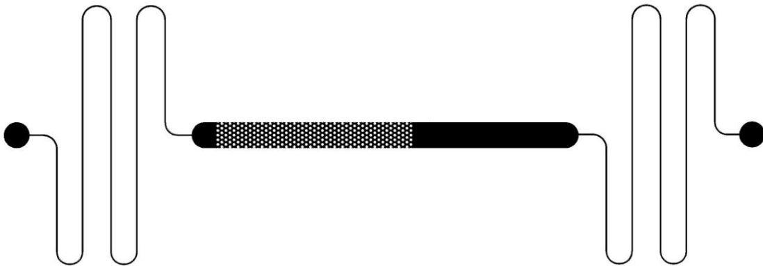
Figure 5: Experimental cell sketch. The black dots at left-end and right-end represent inlet and outlet. The main body of chamber is consisted of two parts: pillar area (hollow dots) and open area (black).
