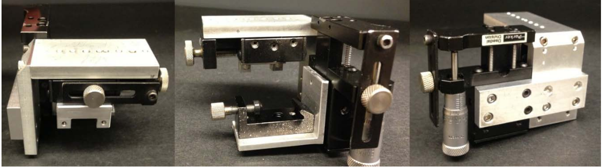
Figure 2.7. Adjustable film mount unit. In the above figure, from left to right, it is displayed from the front, rear and side. This unit was also used to mount the double aperture, shown in Figure 5.X.
