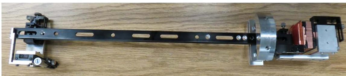
Figure 2.12. Compacted version of interferometer for use on Zebra. The entire assembly without the double pinhole unit is shown.
