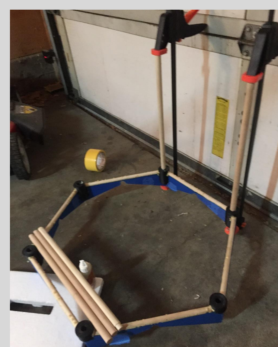
Wooden dowels make up the legs and hoop supports.
