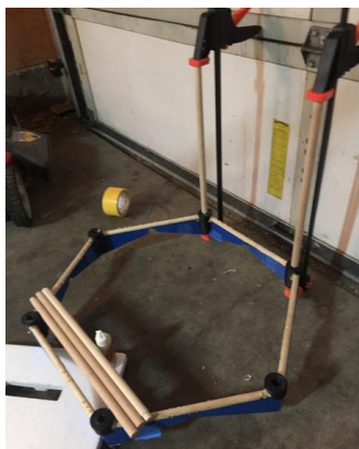
Figure 9: Station Legs being installed to the station leg supports
