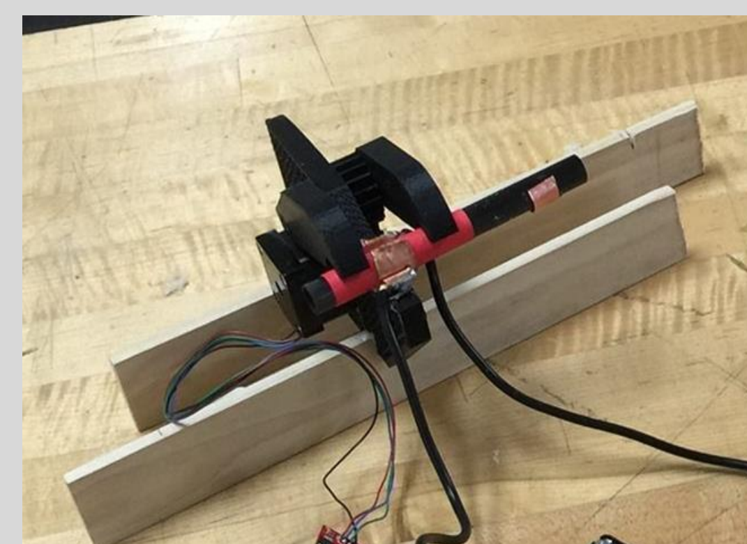
The prototype proved that additional contact pressure was not required.
