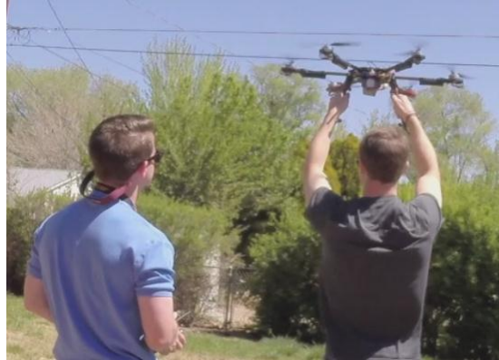
Figure 11: Draining the battery of the UAV prior to testing how rapidly the battery could be effectively charged
