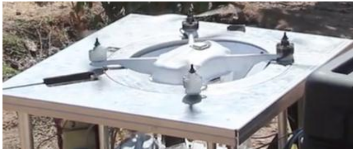
Figure 2: Skycatch battery swap station [1]
