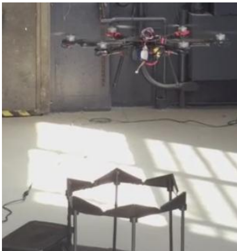
Figure 10: Testing the landing capabilities by manually landing hexacopter on the station
