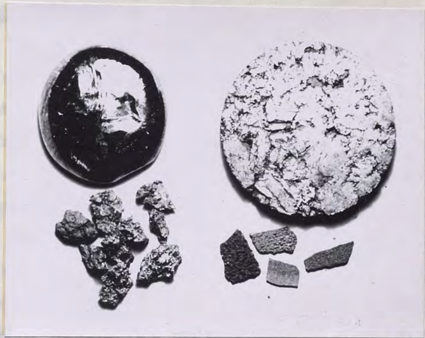
Figure 3. Bottom. (Left) Titanium sponge and (Right) electrolytic manganese used in making alloys. Top. (Left) Titanium alloy button after melting and (Right) titanium alloy compact before melting.
