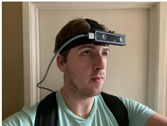
Figure 1. Recording equipment. The T265 measures 6 degree of freedom (6DOF) position of the camera relative to the world, and is worn on the head by a participant over 5 h. The camera plugs into a lightweight laptop worn in a backpack.
