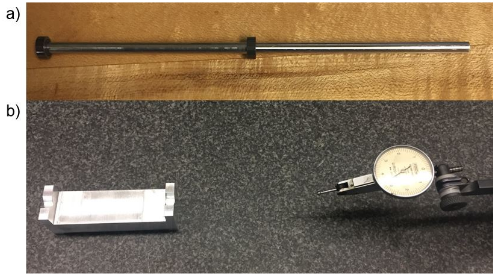
Figure 5.6: a) Shows a Titanium rod with both bearings fixed into place via liquid Nitrogen. b) Shows the jig made to test the TRO of each rod both with and without bearings. The jig holds the rod in the places where the bearings would be. As the rod rotates the dial reads the total deflection of the end of the rod.
