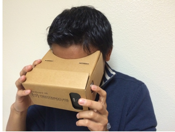
Snapshot 3. The Google Cardboard is a small cardboard box that the user can use with a smartphone to replicate a virtual reality headset.
