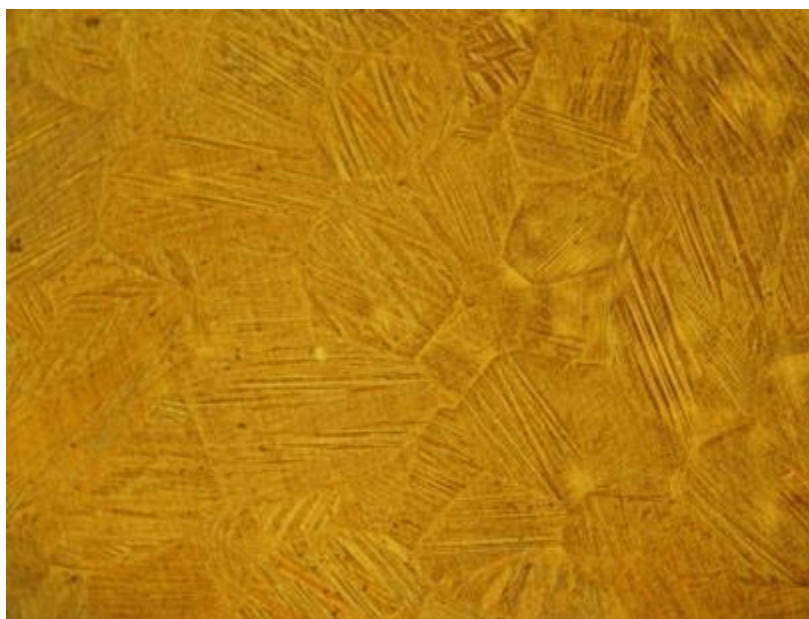
Figure 27. Microstructure of the as-casted eutectic Cu-Zn-Al, x40.
