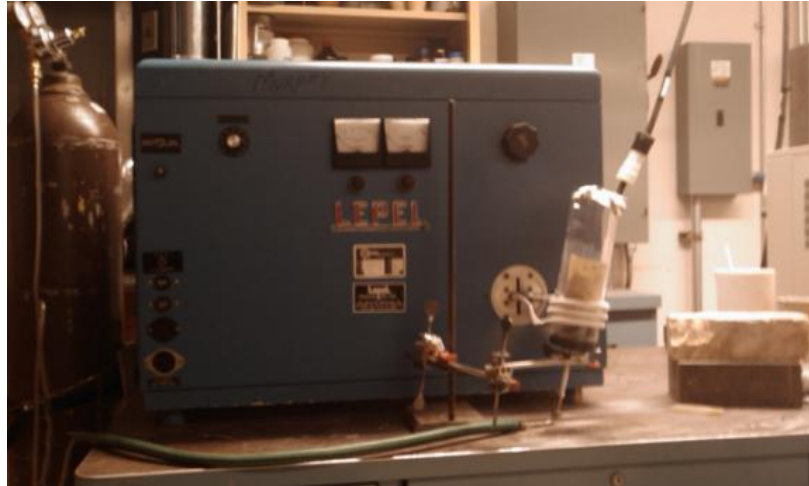
Figure 25. Photograph of the conventional inert gas protection setup for the induction casting.
