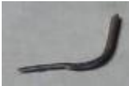
Figure 45. Shape memory effect test of the sample 1 Cu-Zn-Al (Recovering stage).
