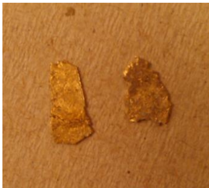
Figure 37. Comparison of the 1 hour heat treatment sample and 4 hour heat treatment sample.
