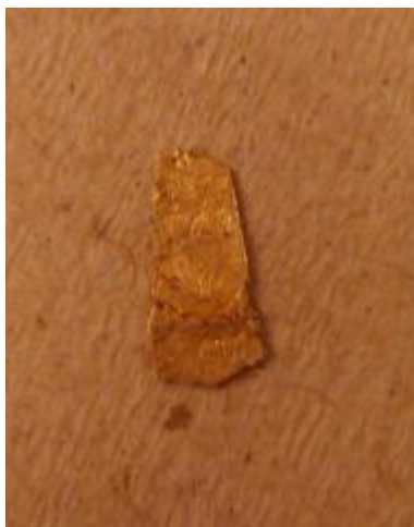
Figure 34. Cu-Zn-Al sample after one hour heat treatment and water quenching.
