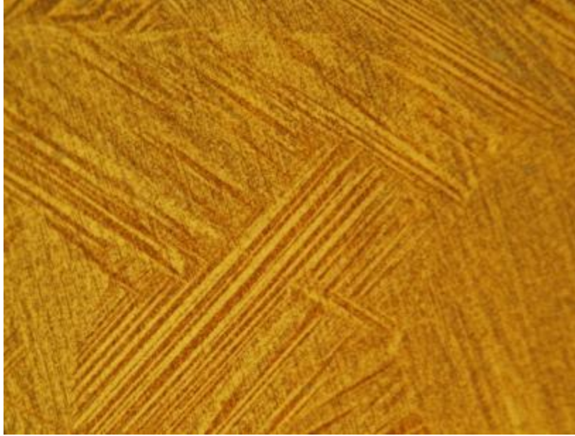
Figure 42. Microstructure of the CZA sample 1 with Cu-Zn-Al, x80.
