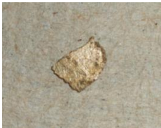
Figure 35. Cu-Zn-Al sample after 2 hour heat treatment and water quenching.
