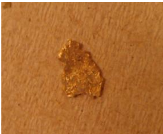
Figure 36. Cu-Zn-Al sample after 4 hours heat treatment and water quenching.
