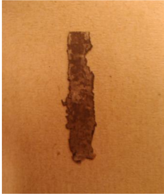
Figure 32. As-rolled Cu-Zn-Al-Mn alloy with a rolling reduction percentage of 3 %.
