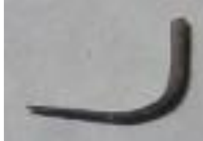
Figure 44. Shape memory effect test of the sample 1 (deforming stage).
