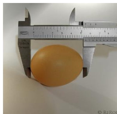
Fig. 6 Sliding calipers in use. Image from ReRod.
