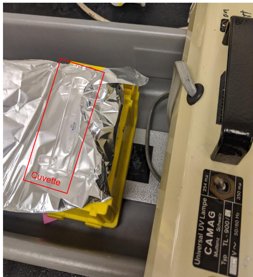
Figure-A-1 Cuvette (37.7 cm 3 ) placed on top of aluminum foil and a pipette box to keep sample close to lamp.
