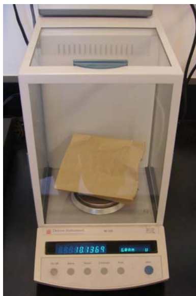
Figure B-5: Litter/duff sample being weighed following oven drying at 50°C for 36 hours.
