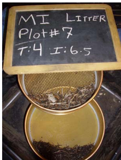
Figure B-4: U.S.A. Standard Test Sieves that were used to sort litter and duff samples from inorganic material such as rocks.
