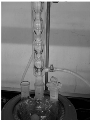
Figure 2.2: The set-up for the reflux process: a triple neck round bottom flask connected with the condenser
