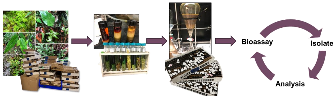
Figure 1.2-1: General isolation process of natural products from plants
