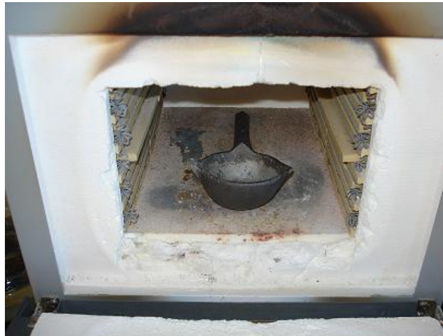
Figure 22 – Ladle inside the Barnstead Thermolyne 48000 furnace prepared to be heated.
