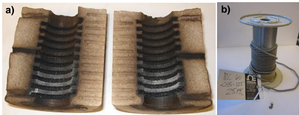
Figure 29 – a) Inside part of the (split in two) ceramic heater showing the metal coil grooves and; b) NIC60 coils used on this task.
