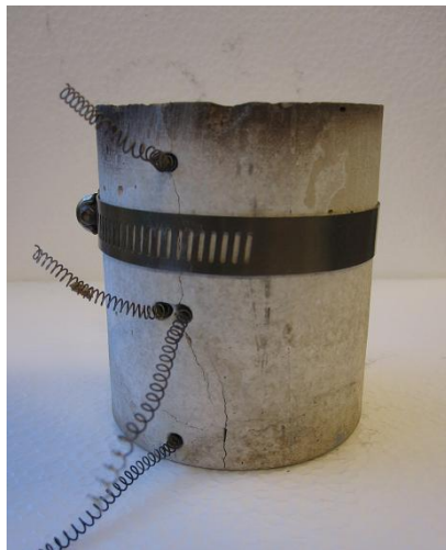
Figure 27 – Ceramic heater showing the heater coils end.
