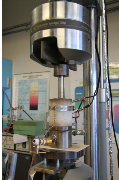
Figure 42 – MTS machine applying pressure on the molten metal during a performance test.
