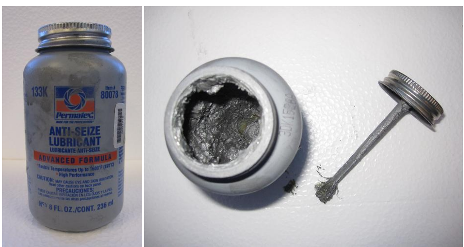
Figure 26 – Anti-seize lubricant used to ease the sample removal from the mold.
