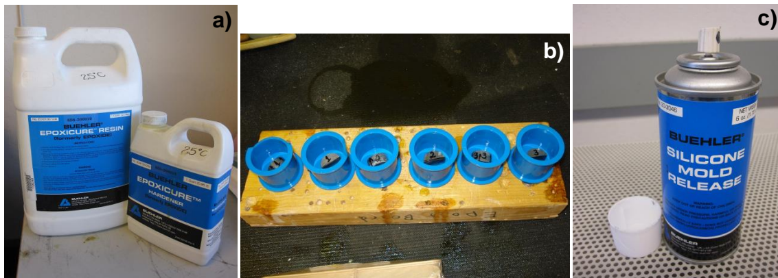
Figure 46 – a) Epoxy and Hardener used to produce the mounting mixture; b) Samples inside the mounting cups ready to be filled with the epoxy and; c) Mold releaser used to facilitate the sample removal from the cups.
