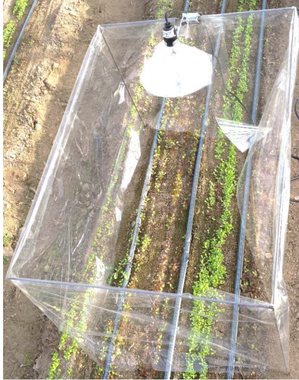
Fig. 2.1. Pictured here is an enclosure used in the study for Chapter 2, specifically for the hoop house experiment. Enclosures were open top and 0.5 m tall, 0.9 m long, and 0.6 m wide. For each enclosure, the lamp was located at the north end to minimize shading of plants. Sides of the enclosures are lined with Type D Mylar that blocks 99% of UV radiation so that plants outside the enclosures are not exposed to additional UV radiation. In the hoop house experiment, green oak-leaf lettuce was grown amongst other greens.
