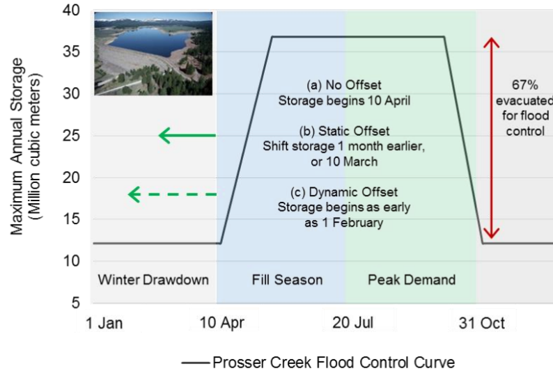
Figure 4. Prosser Creek Reservoir operation simulations. (a) No offset defines the current operations that do not allow for storage before 10 April. (b) Static offset reoperation shifts the flood control curve (black line) to allow for storage one month earlier, or 10 March. (c) Dynamic offset reoperation calculates a fill date annually based on peak inflows, but occurs no earlier than 1 February. Note, 67% of reservoir capacity is evacuated making it susceptible to reduced storage under earlier snowmelt.
