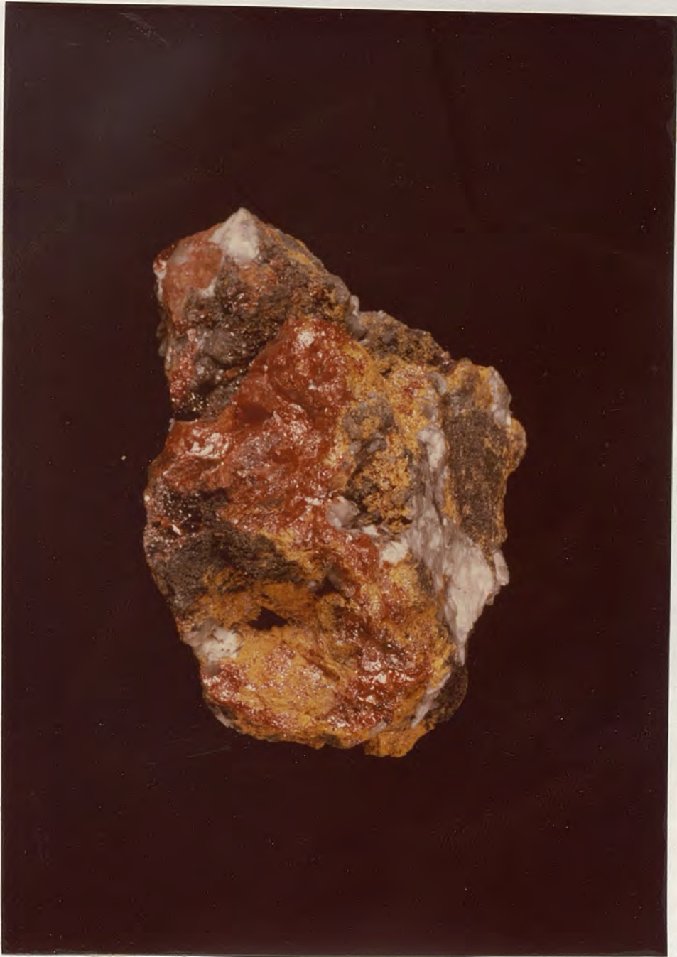
Figure 1. The sample collected from Getchell, Nevada shows the red realgar and the yellow orpiment. The black and white areas are calcium and magnesium carbonate with quartz.
