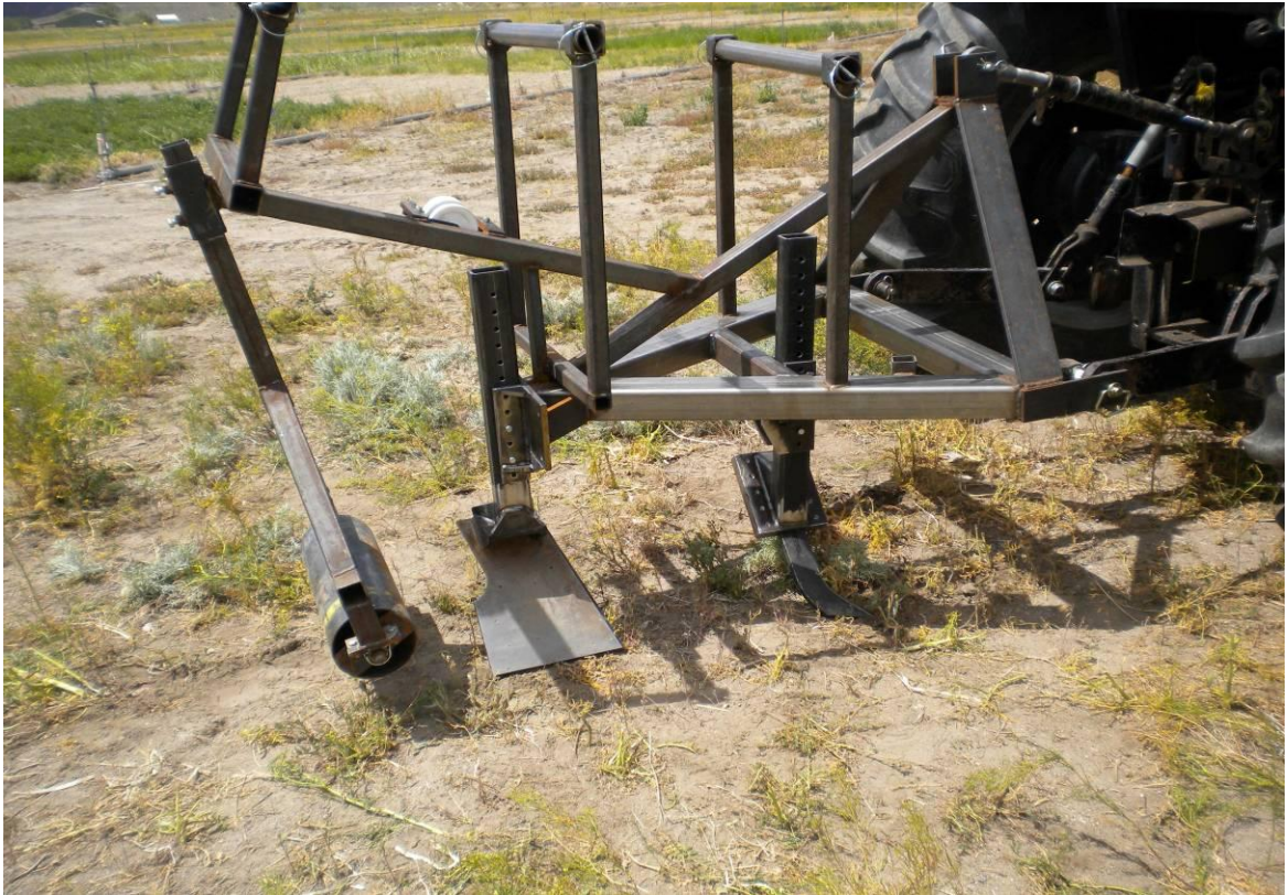
Figure 6.1.1. The plow setup as used to install three cables into the shallow subsurface at the 5C Cottonwood Ranch. The ripper tooth (closest to tractor), cable deploying blade (middle), cement roller (farthest from tractor), and crossbeams to hold spools of cable (top) are shown.
