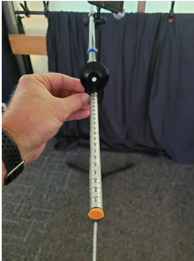
Figure 4: The sliding target used to measure near point convergence for the VOMS prototype. The subject's nose is placed on the orange pad at the end of the slide measure. The subject then holds the sliding target. While focusing on the 14-point target, they move it towards their nose. At the point they see two targets, they are instructed to stop, and the measurement is taken. This is repeated three times. A symptom assessment is taken after the 3rd trial.
