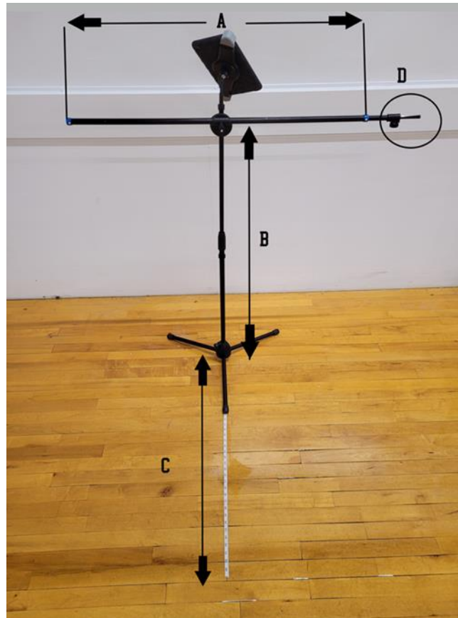
Figure 3: The VOMS prototype target stand. A: a mobile, 36-inch cross piece with white, 14-point targets at each end. This arm is adjustable to a horizontal or vertical position. B: adjustable vertical arm allows for adjustment to the height of the subject's nose. C: measured distance of 36 inches to get the correct distance from the subject's nose to the target stand. D: a sliding measure that extends to the subject's nose for near point convergence measurement. The slide measure has a 30 cm tape on it. An additional sliding target (See Figure 4) is used on the slide measure for the near point convergence test.
