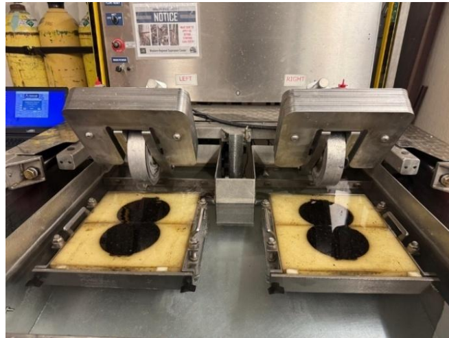
Figure 3.5: HWTT test specimen in Water
