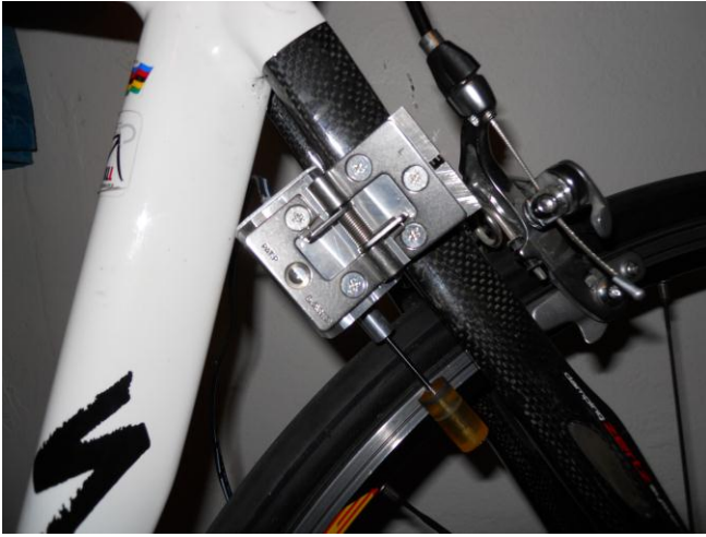
Fig. 16: Generator and mounting bracket assembly mounted onto rear triangle.
