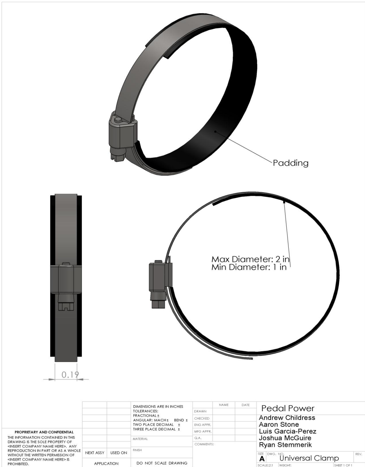
Fig. 9: Universal worm screw clamp with foam padding.
