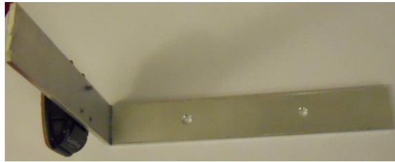
Fig. 16: Water bottle post mounting bracket and quick-release mechanism.
