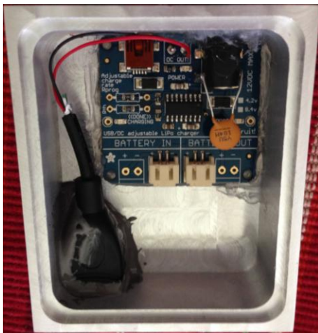
Fig. 13: Electronics pack internal view.
