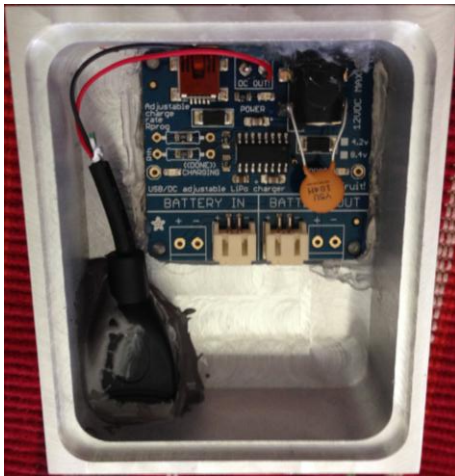
Fig. 21: Electronics pack internal view.
